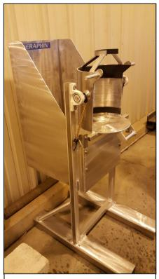
Testing Table/Sink for 5 gallon test measures
