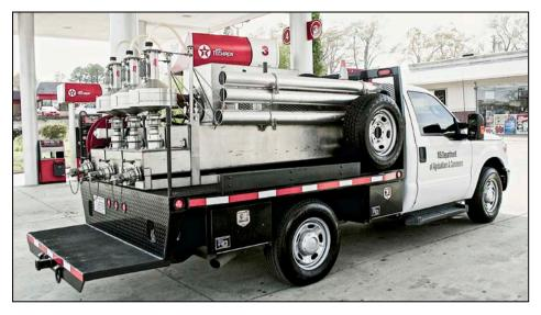
Also modified, were the tubes used to store fill drain hoses. PVC pipes were replaced with aluminum tubing. Petroleum Supervisor Clay Hammons has been instrumental in completing these projects.
