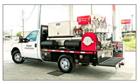
Recent equipment modifications have been made to the flatbed units used petroleum by inspectors. Storage cases holding the 5-gallon hand held measures have been mounted allowing easy access as well as protecting from possible damage. Hose reels have also been added providing easy storage of hoses used with the fuel return system.
