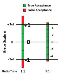
A better way to express this in is terms of compliance rate. Imagine your test data shows compliance of a class of devices as 95% at 1 e tolerance, but you are testing using direct reading. Due to rounding in measuring the error that you are not addressing, 95 % of the instruments are actually within 1.22 e and
