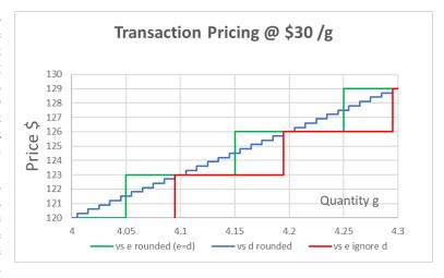
If the user must have a scale with e = d, then it forces them to go to 0.01 g e to service loads at the 1 g level. For that scale 50 e is 0.5 g, and the 1 g loads weighed are near 100 e. Precision scales rarely use 2 or 5 divisions, so capacities
