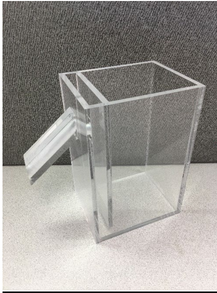
15 Figure 3-7(a). Example of a Displacement Vessel.
