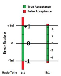
A better way to express this in is terms of compliance rate. Imagine your test data shows compliance of a class of devices as 95% at 1 e tolerance, but you are testing using direct reading. Due to rounding in measuring the error that you are not addressing, 95 % of the instruments are actually within 1.22 e and not the 1.00 e indicated in the compliance data. By increasing the Tol:e ratio to 5:1, 95% of the instruments are accurate within 1.01 e.
